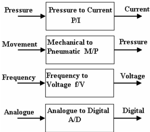
Normally we show them on a block diagram as a box with an input and output with a label to say what it does. Here are some examples.
