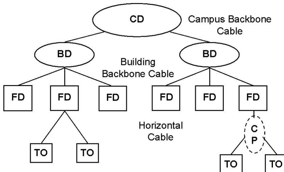
**Figure 1.1:** structured IT cabling according to EN 50173 and ISO/IEC 11801
