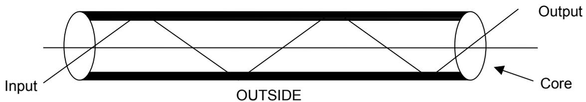
**Figure 5.11:** Light guiding principle of multimode fiber
