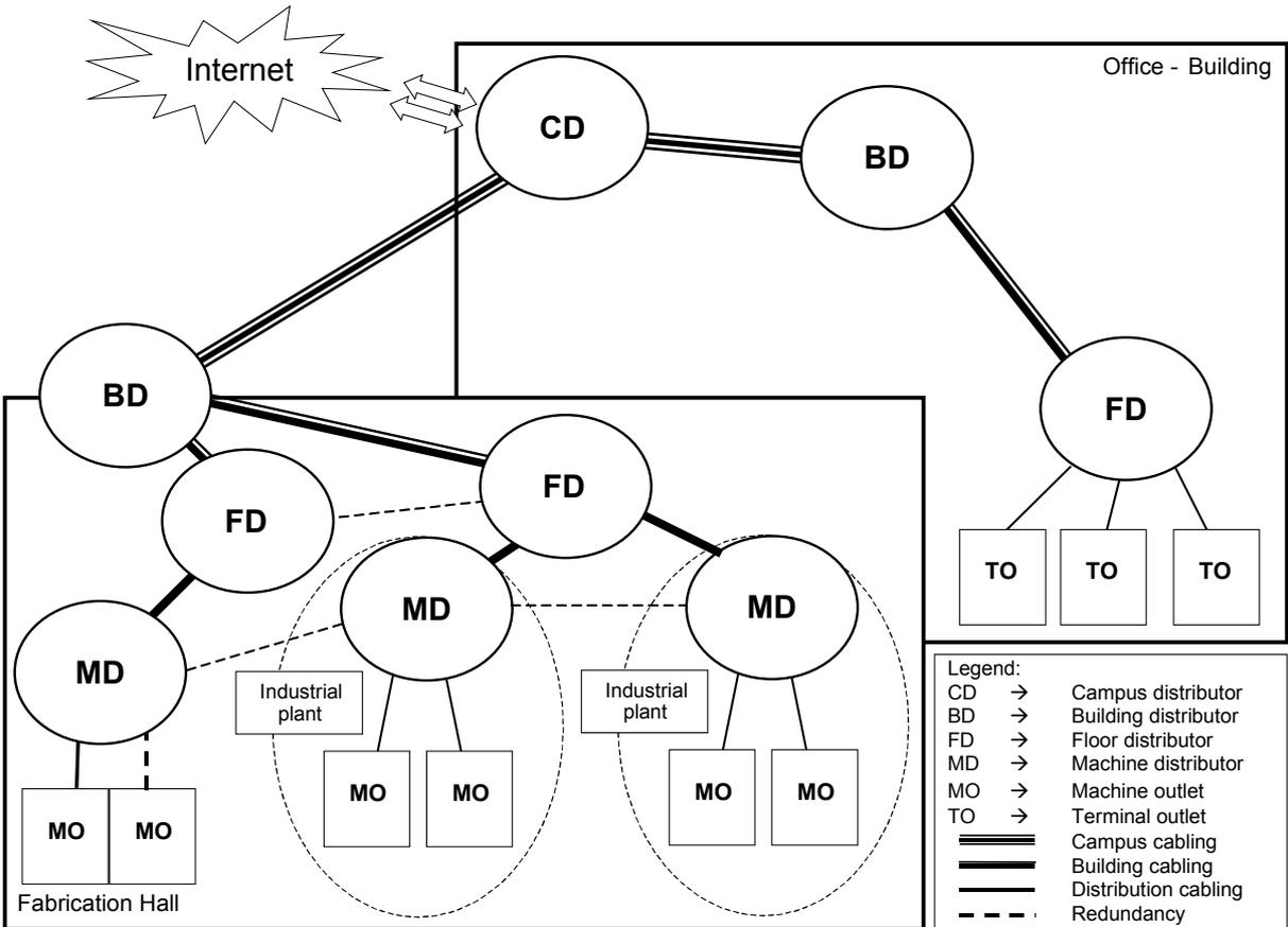
**Figure 2.1:** Example of building backbone cable arrangement at industrial sites
