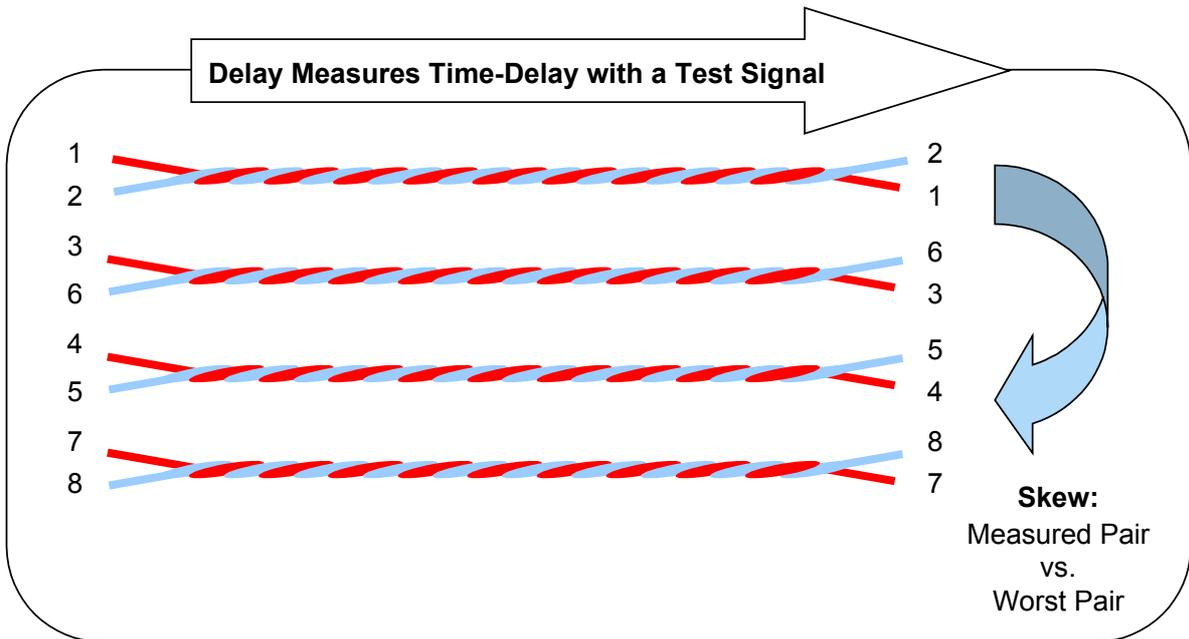
**Figure 5.10:** Delay and skew measurement
