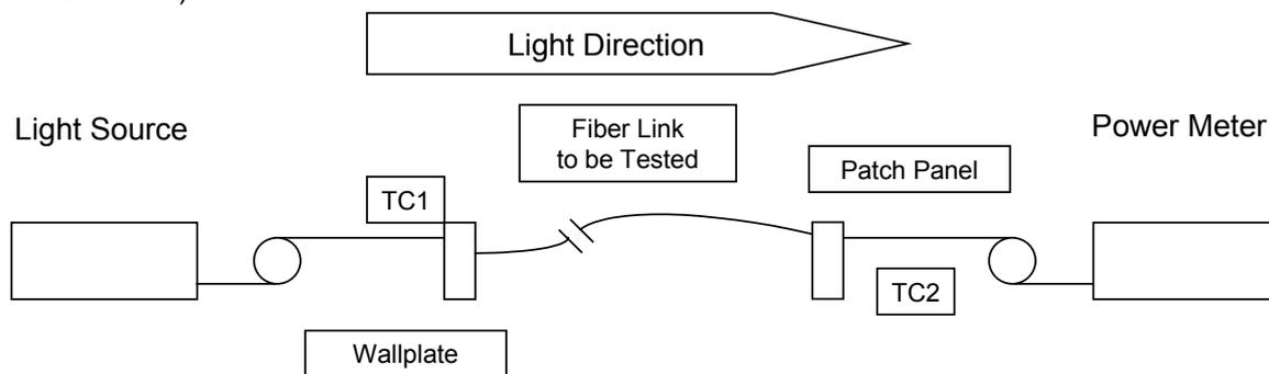
Link Loss = link in the wall loss + two connector losses + Test Cable 2 loss
