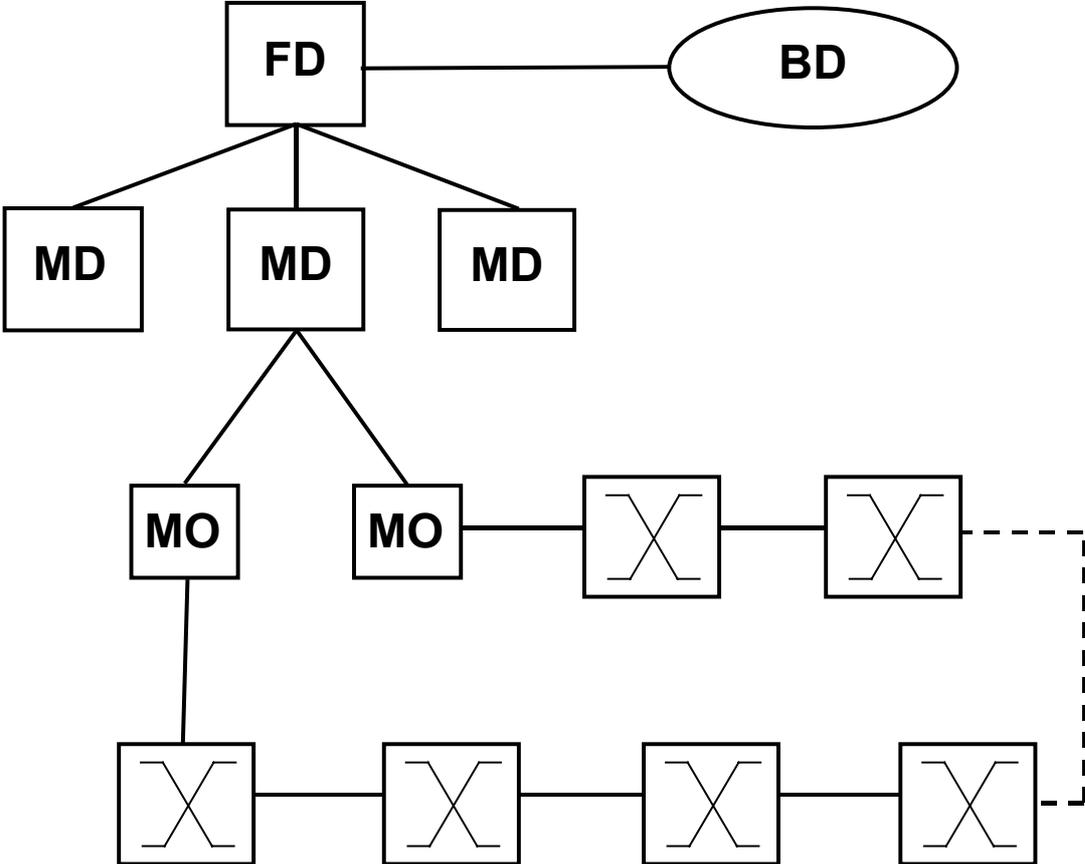
**Figure 2.5:** Ring topology of Ethernet switches connected to MOs
