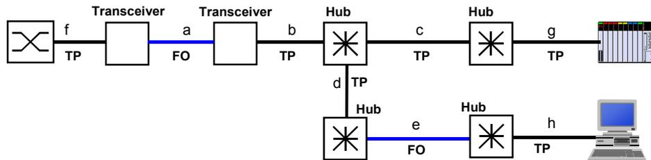
Propagation Equivalence distance f-g:  $2 \times 140\text{m (DTE TP)} + 2 \times 100\text{m (Transceiver)} + 2 \times 190\text{m (Hub)} = 860\text{m}$
