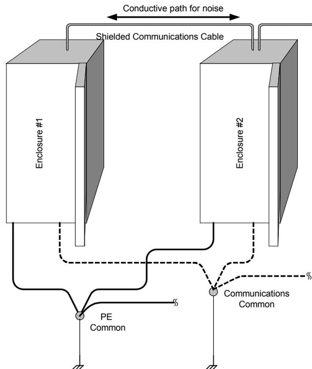
**Figure 3.2:** wiring the grounds in a star ground configuration
