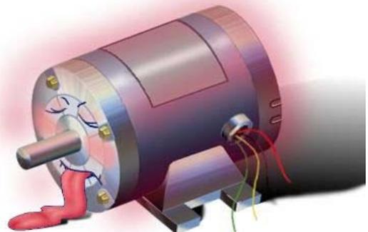
As a rule of thumb, you can generally take a fully loaded Class B insulation motor down to 50 percent speed on constant torque loads without overheating.
